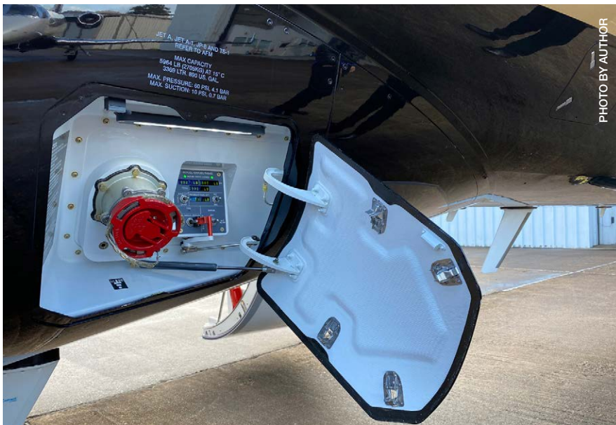
Single-point refueling access.
